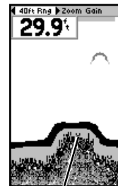
Structure is soft, probably a mud pile
